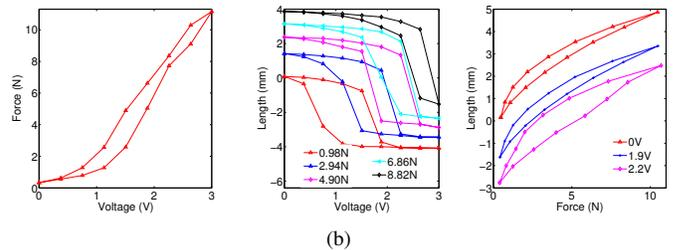
Fig. 1. (a). Three-dimensional and coupled hysteresis in robotic artificial muscles. (b). The experimental  $F - V$  hysteresis (left),  $L - V$  hysteresis (middle), and  $L - F$  hysteresis (right) of an SMA actuator.
